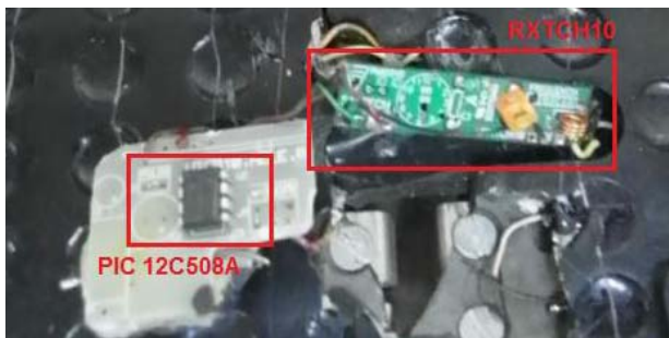
Figure 5 – Printed circuit board with a PIC 12C508A microcontroller and a RF receiver model RXTCH10 [15].
