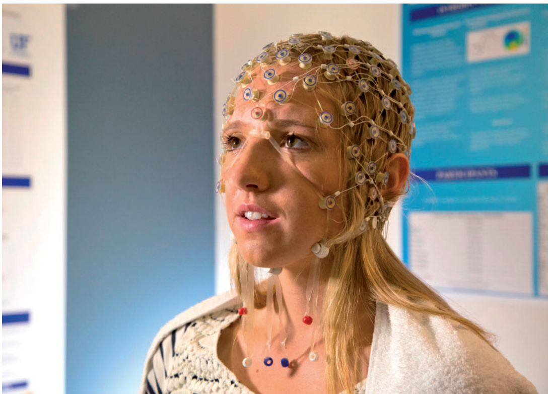
Figure 2. The 128-node HydroCel Geodesic Sensor Net used for recording the EEG.
